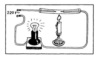
wire to the empty receptacle of the plug, and insulate the connection. Now you have a circuit that is open in only one place, between the ends of the electrodes. Fix the glass tube horizontally. This is easy to do, if the wires are stiff enough, by using plastic insulation; simply bend the wire so that the tube can be supported by it. The preparation is now finished, and it is time to insert the plug into the socket. The bulb will, of course, not light up.
