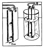
plates to connect them to conductors. Find two identical plastic or wooden spacers no more than a few millimetres thick, and attach them with any water-resistant glue to the metal plates so that they stand parallel to each other.
