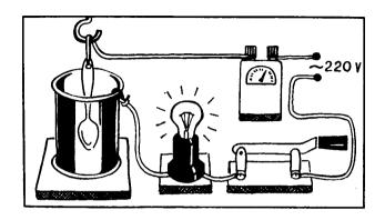
degrease the spoon (you already know how to do this if you conducted the experiments on anodizing aluminium). The spoon will be the first component of the rectifier, and an empty can that is of approximately the same height as the spoon will be the second component.
