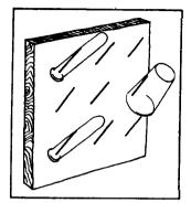
a wooden plank or a sheet of thick plywood up to the heads; then bend the nails at a 45° angle. In order not to injure your hands, wrap the sharp ends with adhesive tape, or put pieces of a rubber tube on them. Just to be on the safe side, you can blunt them with a file. Hang the dryer on the wall, and put a tray under it so that water from the test tubes and vessels will not drip onto the table or floor.
