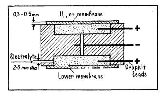
vertically drill in the wall between the cavities a very thin through hole, no more than 0.5 mm in diameter. Make sure that this hole goes through the middle electrode as well!
