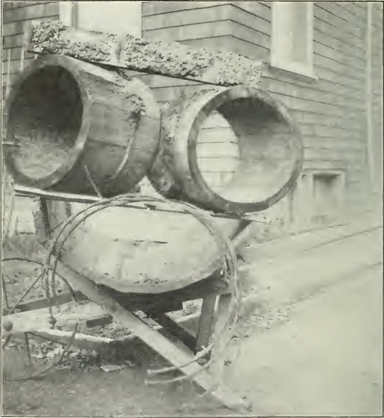
SECTIONS OF WOODEN STAVE PIPE. BANDS, ETC., FROM OUTFALL SEWER AT PALO ALTO, CAL.
