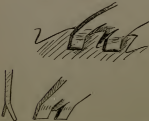
Fig. 99.—Saw Set from Screwdriver.
