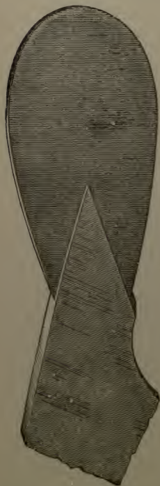
Fig. 45.—Gauge for Circular Saw Teeth.
