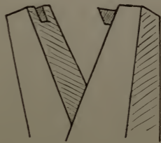
Fig. 97.—Saw Set from Pliers.
